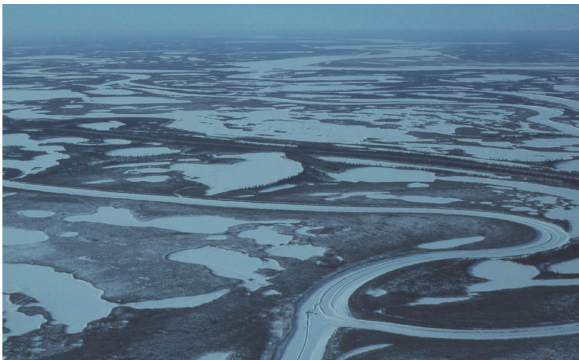
Fig. 1.2 The Mackenzie Delta in winter, showing an ice road built on a river channel (Photo C.R. Burn)
