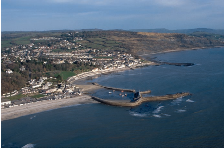
Fig. 22.6 The asymmetrical bays of Lyme Regis. Such bays are typical of the south coast of England caused by diffraction of the dominant south-west waves around headlands and harbor
