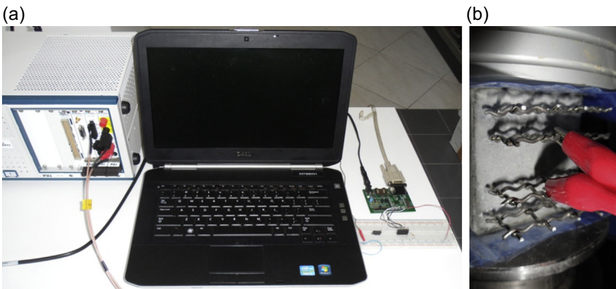
Figure 6.5 Experimental setup: data acquisition system (a), and detailed view of coaxial cables attached to net electrodes of CNTCS (b).
