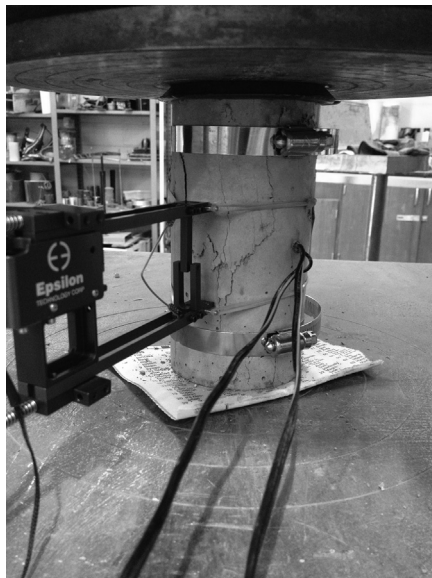
Figure 2.7 Cylinder compression experimental setup.
