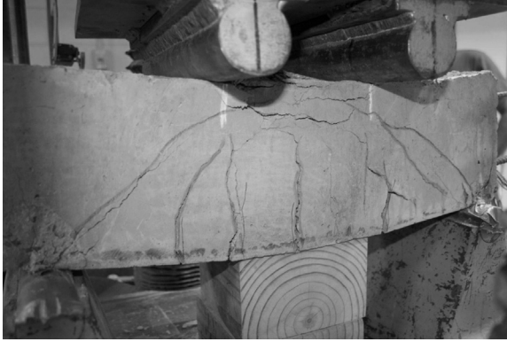
Figure 2.28 Previously tested reinforced concrete beam with flexural and crushing failure modes.
