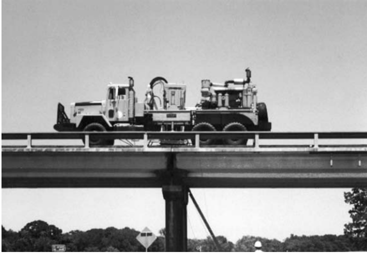
FIGURE 1.44 Vibroseis truck. (Courtesy of Olson Engineering.)
