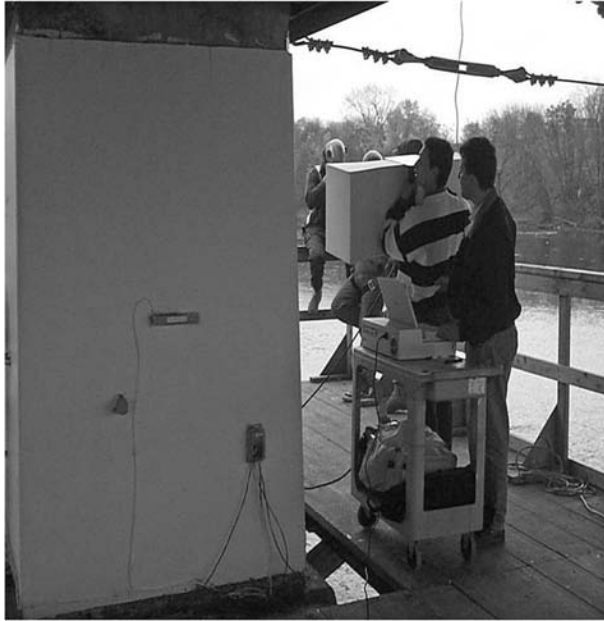
FIGURE 7.24 GPR survey with handheld antenna. (Courtesy of CRC Press.)
