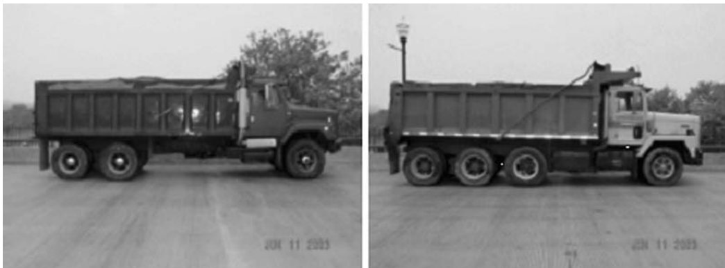
FIGURE 8.47 Three- and four-axle trucks used in the load tests. (Courtesy of New York State Department of Transportation.)
