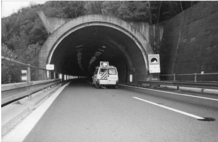
FIGURE 9.41 Scanner mounted on a vehicle (SPACETEC). (Courtesy of CRC Press.)
