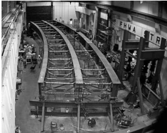
FIGURE 3.14 Curved bridge girder test setup. (Courtesy of CRC Press.)
