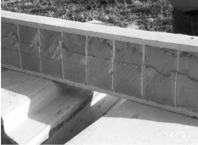
FIGURE 6.17 FRP bridge deck manufacturing: VARTM. (Courtesy of Jerome O'Connor.)
