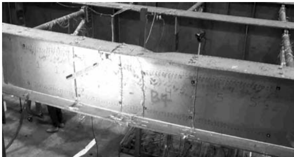
FIGURE 3.15 Component specimen after failure showing top flange buckling. (Courtesy of CRC Press.)
