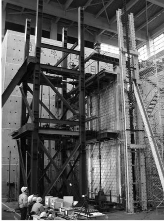
FIGURE 2.17 Seismic testing of shear wall. (Courtesy of MCEER, University of Buffalo.)
