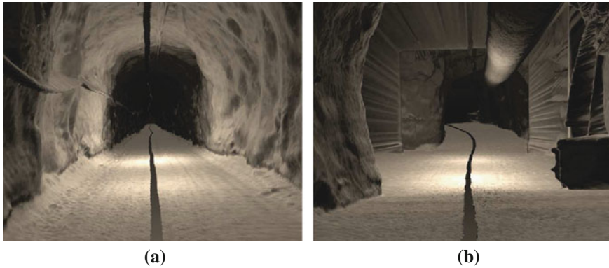
Fig. 5 Two views of the reconstructed surface model of the Northparkes Mine. a A typical section of the decline. The gaps on the floor and ceiling are due to the blindspot between the two vertically-oriented lasers. Electrical cables are seen along the left side wall. b A section of the mine including open ventilation doors and ductwork. Some long surface triangles are seen along the door frame where the surface is essentially parallel to the scanning plane
