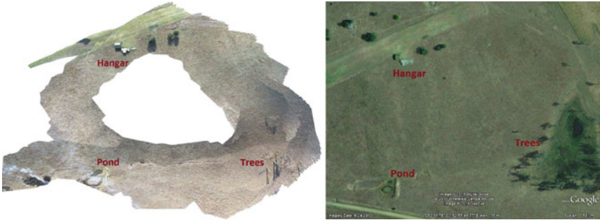
Fig. 7 Left A densely reconstructed ground plane using only camera pose to inform map generation over 879 frames. Right A comparison of the same area on Google Earth, showing qualitative accuracy of the final SLAM estimate
