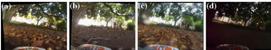
Fig. 1 Visual change in an environment over the course of a day and in varying weather—a dawn, b morning, c rain and d dusk. As well as changing illumination other challenges are present such as motion blur from the jerky motion of the platform when travelling off-road
