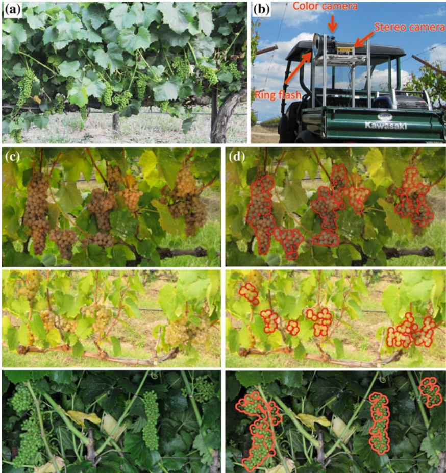
Fig. 1 Photos of the vineyards and equipment from our experiments. Equipment mounted on an aluminum frame fixed on the back tray of a Kawasaki Mule farm utility vehicle. The sensing equipment used is a Nikon D300s color camera facing sideways from the vehicle detecting the fruit, an AlienBees ARB800 ring flash mounted around the lens of the color camera illuminating the scene, a PointGrey BumbleBee2 stereo camera facing back down the row tracking the vehicle motion. Images collected of the vines are processed to detect and measure the vine fruit. a Chardonnay vineyard used in experiments. b Sensors used in experiments. c Raw images. d Detected berries
