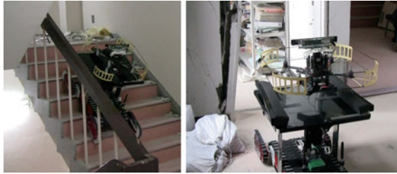
Fig. 3 The Quince ground platform carries the Pelican aerial robot via a landing pad. The aerial robot opens and closes the landing pad via a wireless interface during autonomous take-off and landing
