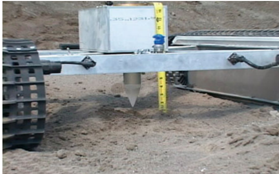
Fig. 3 Icebreaker actuated plow. Conical lexan tip is used to penetrate into the ground [17]
