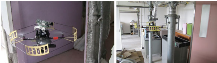
Fig. 5 The aerial robot flies through cluttered regions of the environment that are inaccessible to the ground robot and builds a 3D map that will be merged with the maps made by the ground robot
