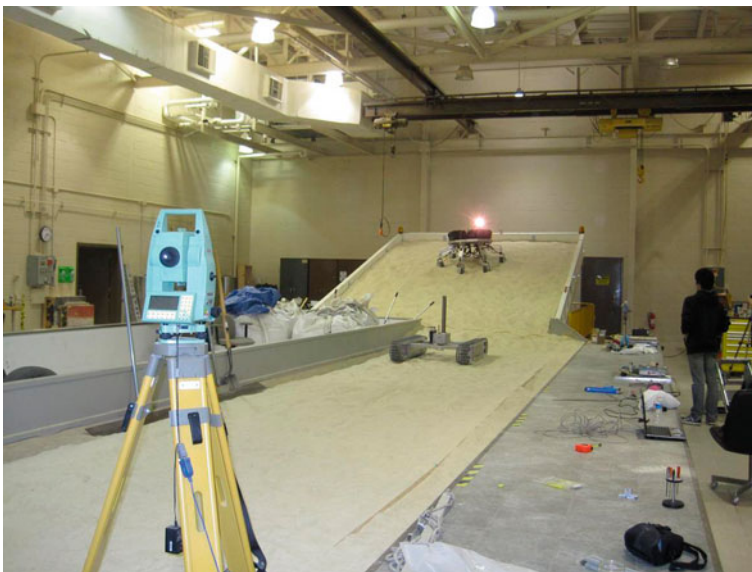
Fig. 6 Test setup with surveying instrument (on the left) and prism (bright spot) mounted on a rover at NASA GRC SLOPE facility
