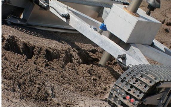
Fig. 2 Icebreaker’s actuated plow. The box contains the motor and pinion for driving the plow into the ground [17]
