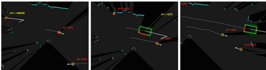
Fig. 10 Result of tracking and identification of moving objects. Circles and squares respectively indicate pedestrians and cars. Although G11 was initially classified as a pedestrian when it was far away from the robot, it was correctly classified as a car when it approached the robot
