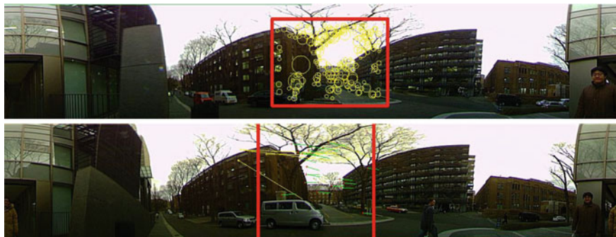
Fig. 14 A result of the angle estimation using FAB-MAP. The upper image is the one selected by FAB-MAP as the one most similar to the lower one. Yellow circles indicate SURF features used in the angle estimations, and green lines indicate the move distances between corresponding points
