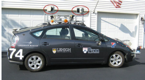
Fig. 3 The mapping vehicle integrated an OXTS RT-3050 GPS/INS for 6DOF vehicle pose estimation, and a pair of roof mounted Sick LMS291-S14 LIDARs (circled red) to capture relative range measurements
