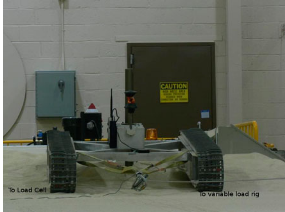
Fig. 9 Draw bar pull test setup with lines going to a load cell and the variable load source
