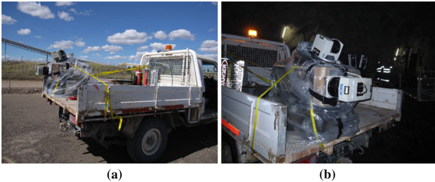
Fig. 1 The vehicle and sensing hardware used for data collection. The plastic sheeting over the sensor cart was used to protect the hardware from mist spray used for dust suppression in some sections of the mine. a The vehicle and sensor cart during setup. b The vehicle and sensor cart inside the mine
