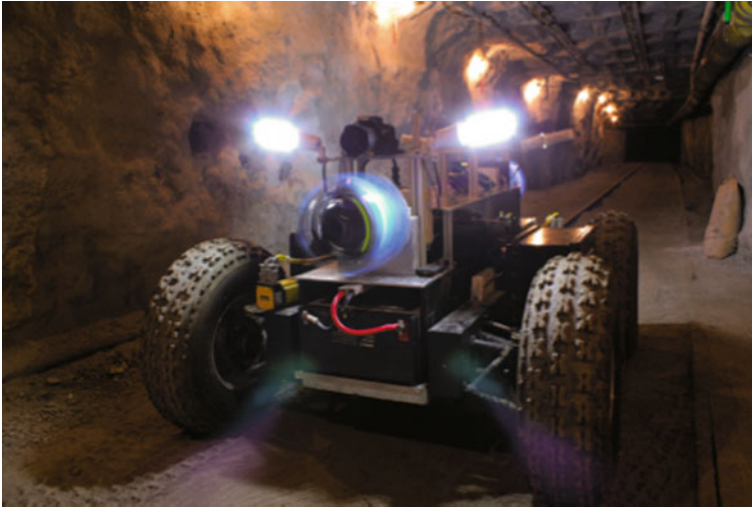
Fig. 2 Cave Crawler platform with spinning SICK in coal mine. Featureless floors, such as the one in this picture, are prevalent throughout this mine and provide little additional information to aid scan matching. Picture by Uland Wongg
