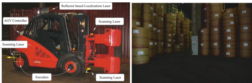
Fig. 4 Left The industrial truck used in the MALTA project. The truck is retrofitted with an AGV controller. The bottom lasers are used as safety sensors and in this work also for landmark detection. Right Stacked paper reels waiting to be loaded and one of the concrete pillars
