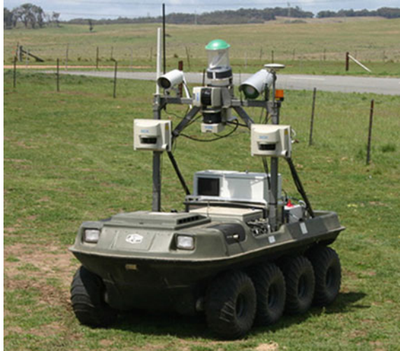
Fig. 1 The CORD UGV employed in this research. The sensor suite can be seen, attached to a rigid frame
