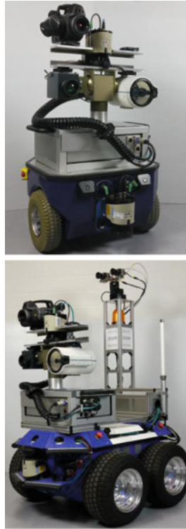
Fig. 9 Inspection module on Neobotix MP-S500 ( top ), MobileRobots Seekur Jr. ( bottom , courtesy of Human-Machine Systems Engineering, University of Kassel)
