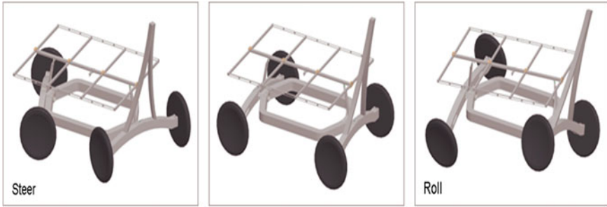
Fig. 3 Zoë's axles are free to rotate in both the steer and roll angles
