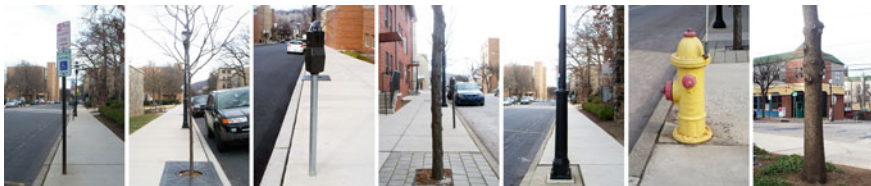
Fig. 4 Instances of the 7 landmark classes. Landmarks were classified and tracked based upon geometry and reflectivity. Detected landmarks could be reliably associated with their respective classes, which prevented data association errors in our experiments
