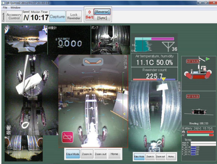
Fig. 7 Improved operator console screen for Quince 2. Status indicators for information such as the amount of cable remaining, temperature, and wireless signal strength, and some alert signals were added
