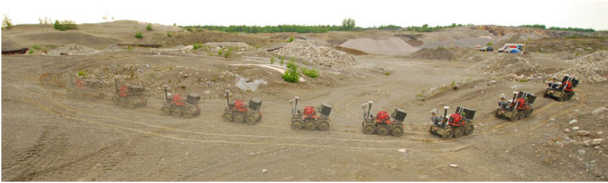
Fig. 1 Panoramic view of the planetary analogue test site in Sudbury, Ontario, Canada. Located inside a gravel pit, the site was chosen for its lack of vegetation and three-dimensional character. Our field robot can be seen traversing the site here in the daytime, although our test data were gathered at night
