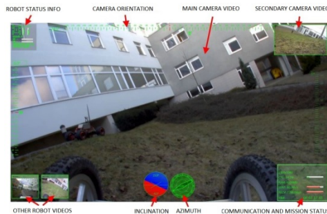
Fig. 5. The screen of the user interface of the Cassandra operator system
