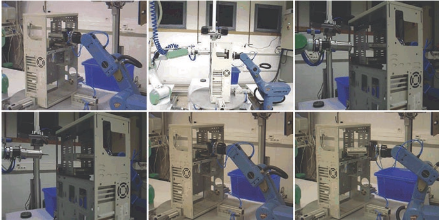
Fig. 3.15 Multi-sensorial cooperative robots—demonstrate removing CD drive [25]
