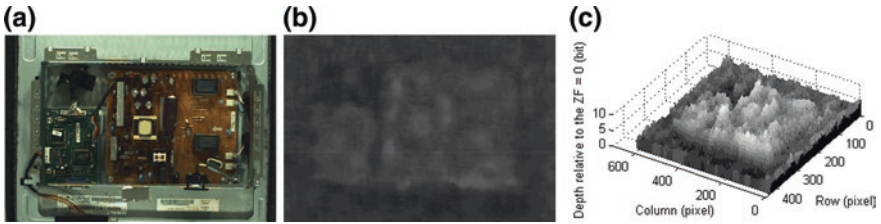
Fig. 4.21 State change—original condition (flagged images). a Colour image. b Depth image. c 2.5D depth map
