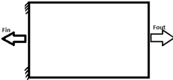
Fig. 2. Design domain with load scheme for force inverter
