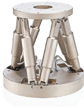
(a) CAD rendering of a Gough-Stewart platform, a general hexapod with 6 degrees of freedom and 6 actuators.
