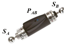
Fig. 1. A ball bar with two master balls and one displacement sensor
