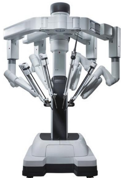
**Fig. 15.6** da Vinci Xi patient-side cart interface with one-button setup and targeting system. ©2016 Intuitive Surgical, Inc.
