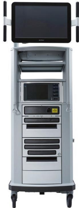
the assistant and OR staff. The vision cart also has integrated energy for EndoWrist instruments that are capable of delivering energy. The generator manages mono and bipolar energy by setting the desired tissue effect.
