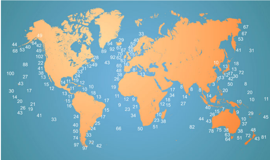
Fig. 11.2 Map of wave power per unit length (kW/m) worldwide [7]
