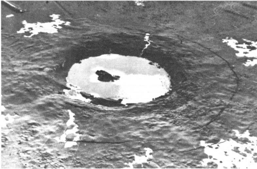
Figure 5.9 Panoramic view of Snowball crater showing central uplift in a moat of groundwater. Diameter of crater is 87 m (after G.H.S.Jones).
