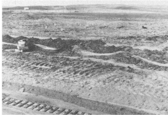
Figure 5.17 Sections of small-wave length folds that developed in tarmac paths, outside the crater rim (after G.H.S.Jones).
