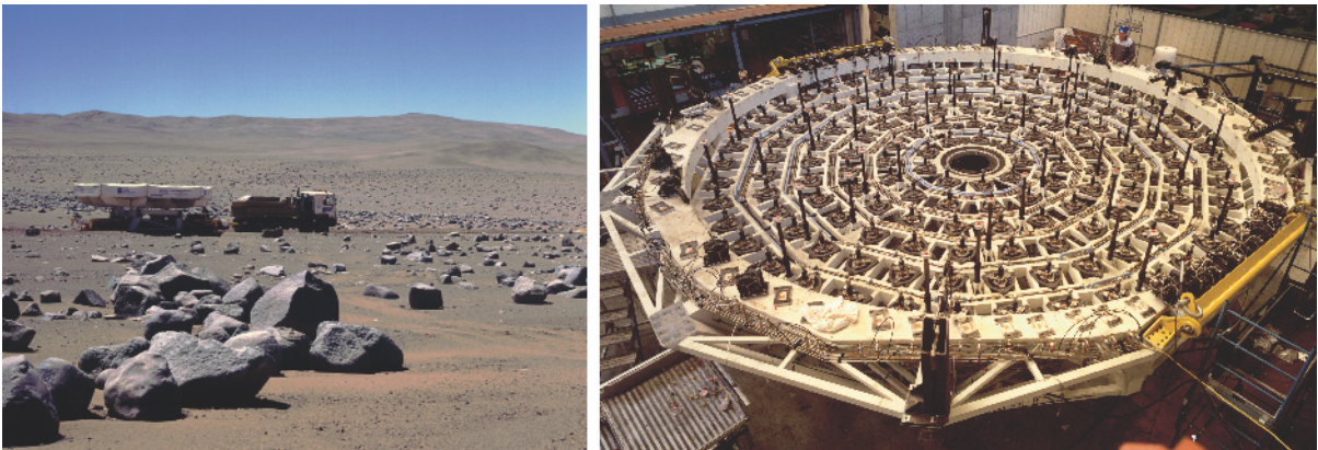
Fig. 1.30. Left: Transport of one of the VLT mirrors from Antofagasta to Paranal. The route passes through an extremely dry desert, and large parts of the road are not paved. The VLT thus clearly demonstrates that astronomers search for ever more remote locations to get the best possible observing conditions. Right: The active optics system at the VLT. Each mirror is supported at 150 points; at these points, the mirror is adjusted to correct for deformations. The primary mirror is always shaped such that the light is focused in an optimal way,
