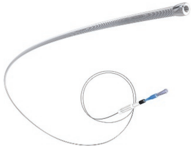
Figure 31.15 The CrossBoss coronary chronic total occlusion crossing catheter (Boston Scientific, Fremont, CA). The CrossBoss is designed to facilitate passage of coronary guidewires via either the true lumen or a subintimal pathway. The rounded tip reduces risk of perforation. A hydrophilic coated, multiwire coiled shaft provides precise turn-for-turn response. The Fast-Spin torque device allows rapid rotation of the catheter to facilitate crossing.
