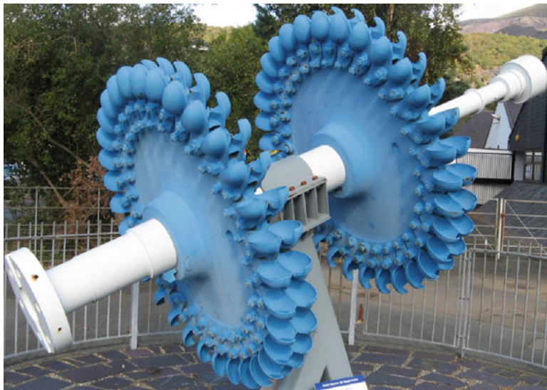
Fig. 1.3 The runner for a Pelton turbine (Courtesy GWEFR Cyf)
