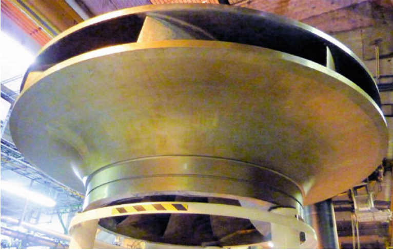
Fig. 1.2 Photograph of a modern Francis turbine runner showing the intricate geometry of the inflow and outflow vanes (Courtesy First Hydro Company)
