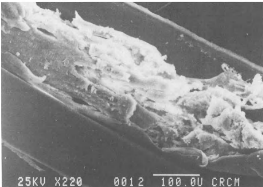
Figure 13. (A) Scanning electron microscopy of the tip of the catheter shown on Figure 12B. (B) Scanning electron microscopy of an obstructed IP catheter.
