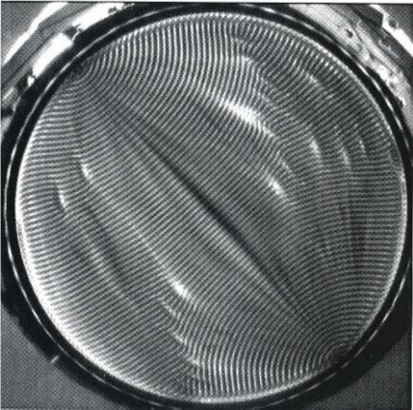
Fig. 12.1. Primary striped wave pattern formed at high viscosity \nu = 1.0 \text{ cm}^2 \text{ s}^{-1} and frequency f = 45 \text{ Hz} at large aspect ratio (from [2]).
