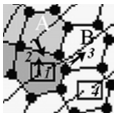
Fig. 9.8. The mechanism of the pentagon formation: Glide motion (steps 1 and 2) of the original dislocation denoted by A and climb motion (step 3) of the new dislocation B . The direction of the movement is indicated by arrows [32].
