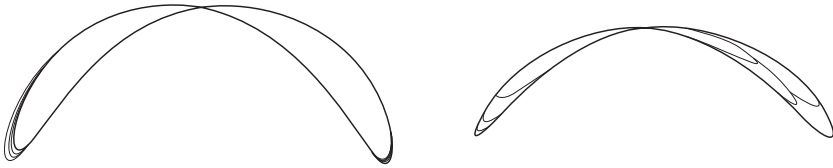
Fig. 2.11. Physical limit cycle and transients, in Bourrières' experiment [36].
