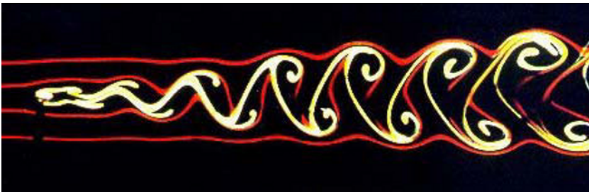
Fig. 10.3. Visualization of the vortex behind a circular cylinder (Courtesy of T. Leweke).
