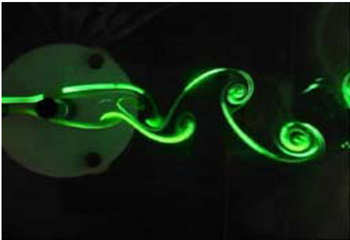
Fig. 11.2. Laser-induced flurosceine view of vortex emission [14].
