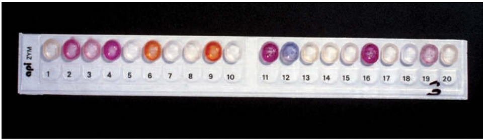
Figure 6.36. An API zym strip after inoculation, incubation and the addition of reagents. The organism is the type strain of Ren. salmoninarum .
