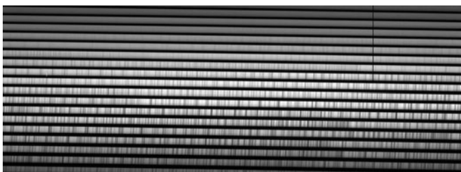
Fig. 3.8 A spectrum of molecular iodine taken with an echelle spectrograph. Each band represents a different spectral order and redder wavelengths are to the right and bottom. The iodine spectral lines begin to become visible at about 5,000 Å
