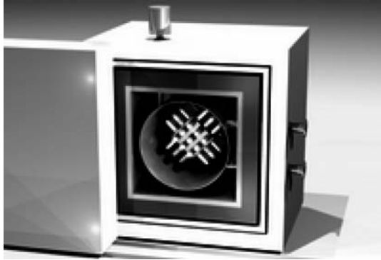
Fig. 3. XMASS prototype detector. 100 kg liquid xenon and 54 low-background PMTs are used. PMTs are attached to the 30 L OFHC chamber through 5 mm thickness \text{MgF}_2 windows. They are put into a heavy shield in a clean room. The XMASS prototype detector is located in Kamioka Observatory, ICRR, Univ of Tokyo, in Kamioka mine.
