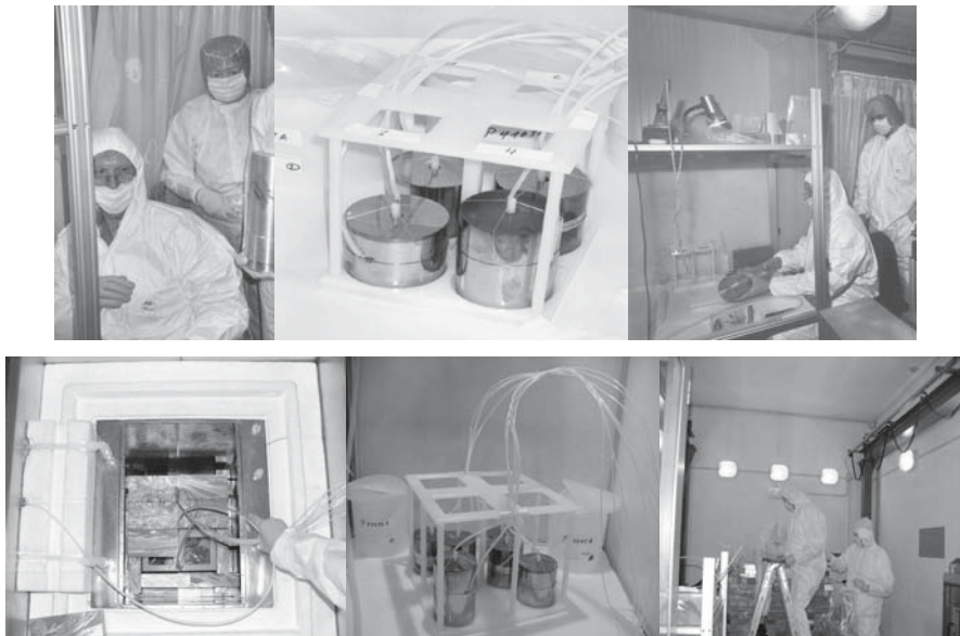
Fig. 1. Upper part – left and right: Taking out the crystals from the transport dewars and fixing the electrical contacts in the clean room of the GENIUS-TF building – from left to right: H. Strecker, I. Krivosheina, H.V. Klapdor-Kleingrothaus. Middle: The first four contacted naked Ge detectors before installation into the GENIUS-TF setup. Bottom part – left and right: View from the top of the new GENIUS-TF-II setup in the more Radon-clean beta-beta room, during installation in October 2004. Middle: The first six contacted naked Ge detectors.
