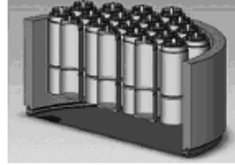
37 two-inch PMT readout set for good position sensitivity and 3-D event reconstruction. Alternative charge readout or low activity devices are being studied
