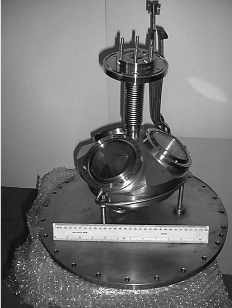
Fig. 2. The Zeplin-1 design: a pure LXe scintillator with 4 kg active mass.
