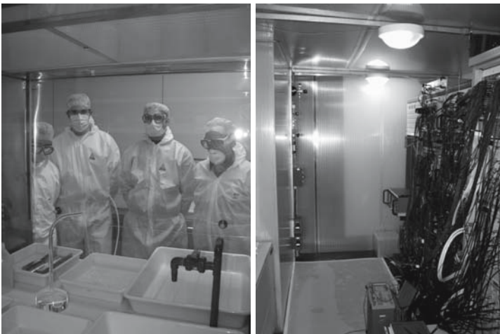
Fig. 2. Left: During the chemical etching of the metallic surfaces in clean room. Particular dedicated protocols have been defined and followed; after the etching the materials have been sealed in HP Nitrogen atmosphere Right: Partial view of DAMA/LIBRA set-up.
