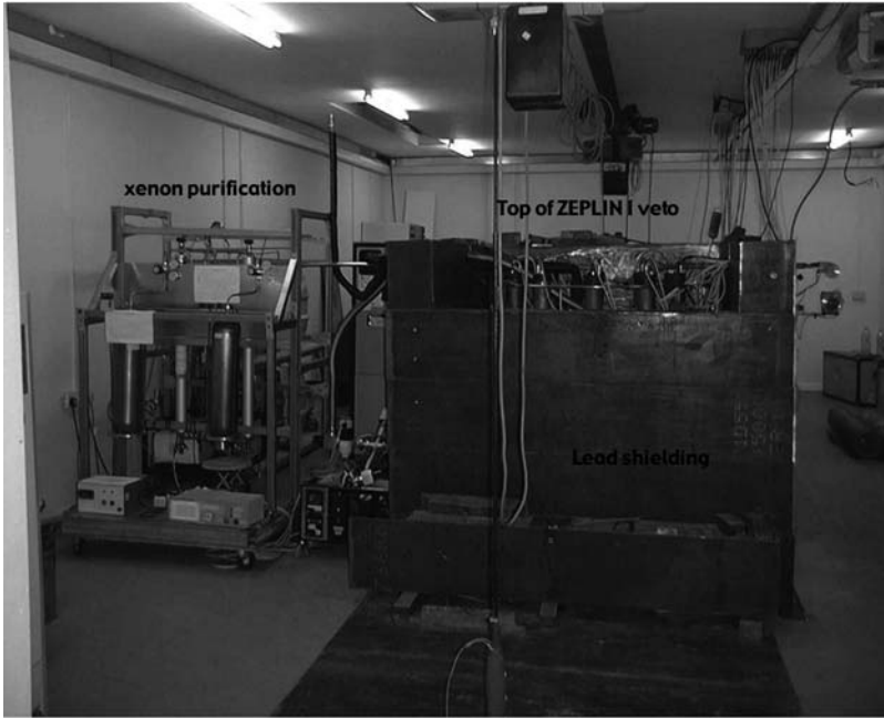
Fig. 5. Zeplin-1 underground, surrounded by its lead shielding.
