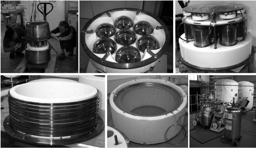
Fig. 2. Internal target installation. Figure shows completed PTFE cone assembly, PMT layout, PMT assembly, field shaping ring assembly with two resistor chains shown, general overview of the ZEPLIN II detector, associated infrastructure and closing up of the target.
