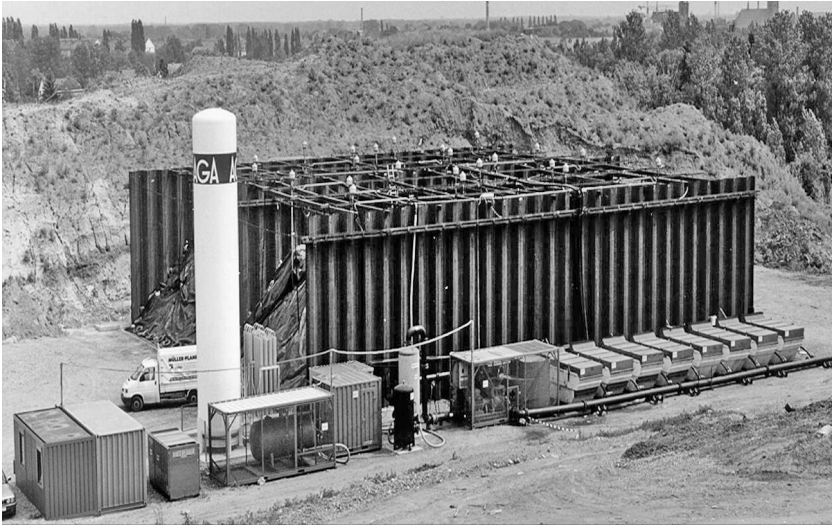
Fig. 11-37 Full-scale test rig for mechanical-biological waste treatment with separation of non-uniform material into specified fractions (Eschkötter, 2004)
