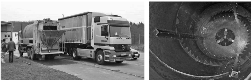
Fig. 11-36 Mixing drum with integrated jet cutting device. Cooperative research project for the integration of jet cutting in the drum. Successful industrial application (Nassour et al. , 2002)
