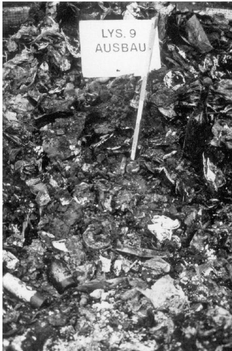
Fig. 8-7 Wastes during removal of the highly chemically contaminated anaerobic municipal waste (Lys. 9) (AUSBAU = REMOVAL)
