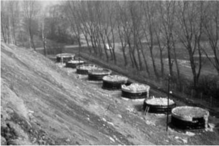
Fig. 2-4 Test facility on the Braunschweig-Watenbüttel landfill, Building stage 1, eight landfill types as lysimeters including the most important sampling arrangements for solids and leachates (Lys. 9 (type 1) and Lys. 10 (type 6) followed as highly contaminated stages 3 years later)
