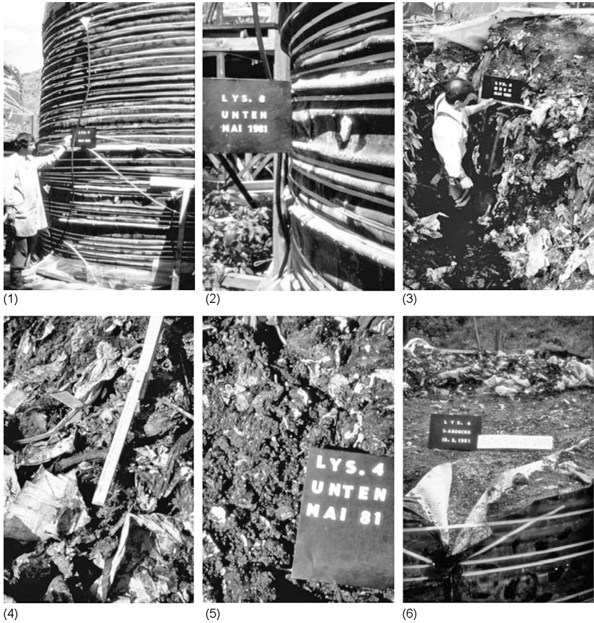
Fig. 2-11 Dismantling of selected lysimeters (Lys. 1, 4 and 8). (1) Checking of the load-bearing outside wall (Lys. 4); (2) waving of the outside skin due to sagging (folds curve inward, since the steel reinforcement of the outside skin does not stretch) (Lys. 8); (3) cut through a deposit for sampling (Lys. 8); (4) typical profile of a sludge-free municipal waste after 5 years of predominantly anaerobic degradation (Lys. 1); (5) typical profile of a sewage sludge waste mix after 5 years of anaerobic degradation (Lys. 4); (6) proof of efficacy of leachate sampling arrangement ( \frac{1}{2}h , Lys. 4) until dismantling (no deposition or incrustation inside the deposit)
