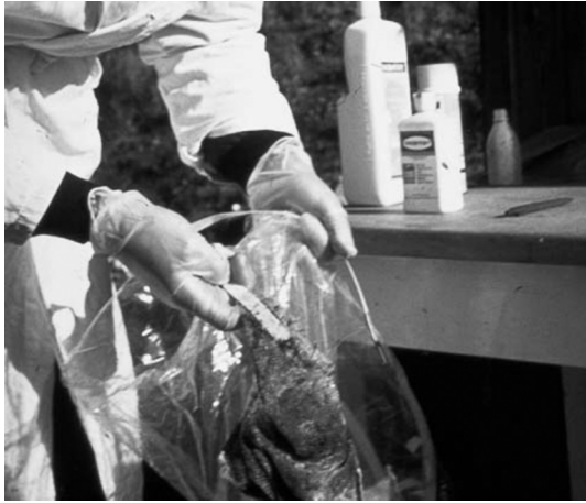
Fig. 2-9 Gauze bag for insertion of bacteria carriers and ampoules to be placed directly in fresh waste
