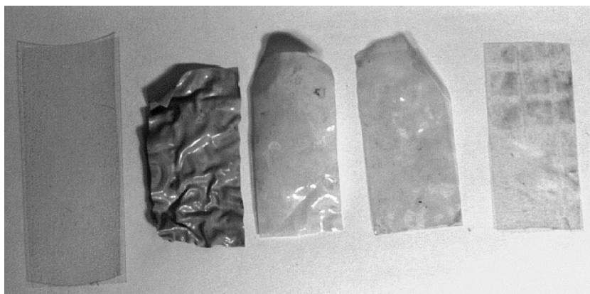
Fig. 9-12 Visible changes of soft PVC packing film (from left to right): (1) initial material fresh from the factory, (2) after aerobic ageing (approx. 80°C), (3) after aerobic/anaerobic ageing (approx. 60°C–80°C alternating), (4) after anaerobic ageing (60°C), (5) ageing in a real biological waste treatment in aerobic operation (50°C)
