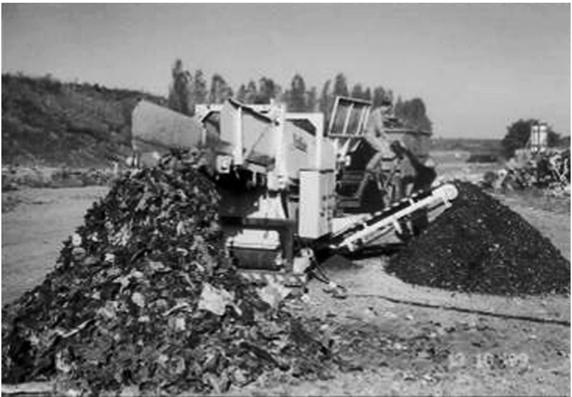
Fig. 11-38 Separation of aerobically stabilised residual waste. Shredder (background) with attached disk separator (front) of the EuRec Technology GmbH (Eschkötter, 2004)
