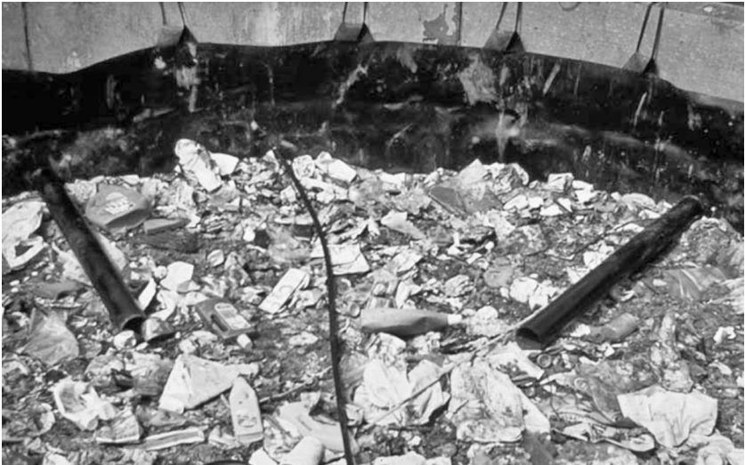
Fig. 2-8 Installations to take material and gas samples from the lysimeters (Lys. 1–10)
