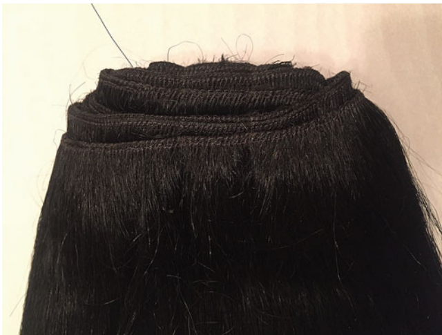
Fig. 5.6 Extensions (“hair tracts”) are created using machines that sew small pieces of hair together onto a strip (tracts)
