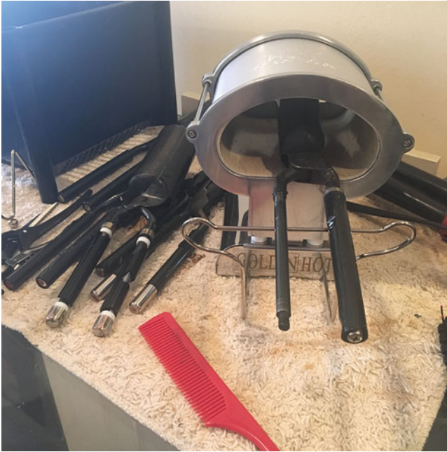
Fig. 3.1 Marcel stove, a specially designed stove for heating hot combs
