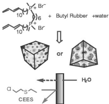
Fig. 23 Selective vapor transport with a cross-linked Q_I -phase LLC-BR membrane ( gray areas = hydrophobic organic domains; white areas = aqueous domains). Reproduced with permission from [170]. © 2006 by Wiley-VCH
