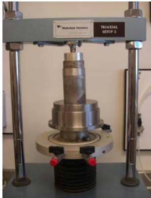
Figure 4. In-place static compaction of ring-shaped SM sample in triaxial frame
