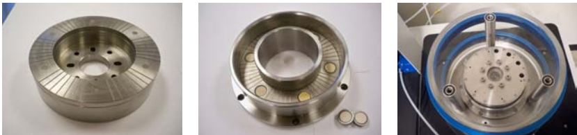
Figure 2. Upper platen (shown upside down), lower platen, and bottom torsional gear
