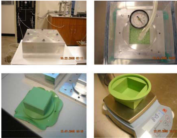
Figure 3. Custom-made mold and fabrication process for cubical latex membranes
