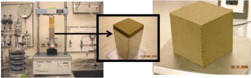
Figure 6. Static compaction process and typical statically-compacted specimen
