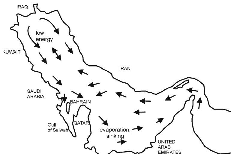
Fig. 4.15 Residual circulation (From Hunter 1983a and Lardner et al. 1993; ship drift data. Permission by Elsevier)
