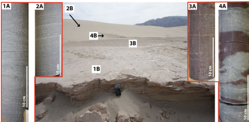
Fig. 5.5 Close lateral changes in aeolian sediment 1–4 core material of the subsurface area in NW Germany, 1 damp sandflat deposit, 2 aeolian dune base deposit, 3 pond deposit, 4 lake or pond margin deposit. I–IV closely spaced lateral changes with dune successions (dry sandflat—aeolian dune), pond and damp-wet sandflat. Arabic numbers of the sedimentary facies in the cores correlate with roman numbers of the sedimentary facies in the modern analogue
