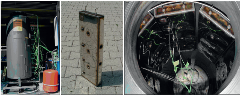
Fig. 9.59. Outside view of the test storage with temperature sensors, PCM module, and inside view with PCM modules fixed at the top of the storage (pictures: ZAE Bayern).
