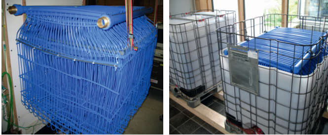
Fig. 9.45. Left: heat exchanger made from capillary tubes with distribution pipes. Right: storage containers made of HDPE with the heat exchanger inserted (pictures: ZAE Bayern).
