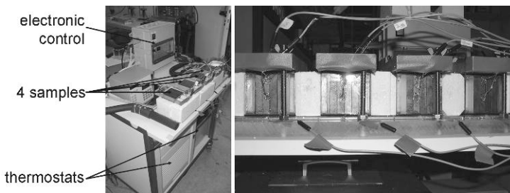
Fig. 3.31. Experimental setup for automatic heating and cooling of four samples and recording of the temperature over time (pictures: ZAE Bayern)
