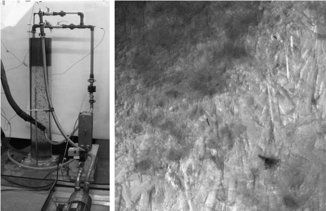
Fig. 5.16. Experimental setup of a direct contact system and PCM-oil mixture in the solidified state (pictures: ZAE Bayern)
