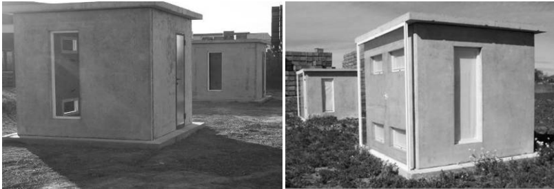
Fig. 9.13. Left: test buildings with walls from regular concrete and from concrete where microencapsulated PCM was added. Right: test buildings with additional trombe wall (pictures: University of Lleida).
