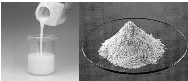
Fig. 2.32. Microencapsulated paraffin produced by BASF, on the left as fluid dispersion, and on the right as dry powder (pictures: BASF).
