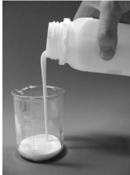
Fig. 9.43. Slurry based on microencapsulated paraffin (picture: FhG-ISE).
