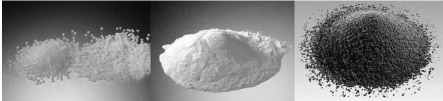
Fig. 2.23. Composites developed and commercialized by Rubitherm Technologies GmbH. From left to right: compound PK, powder PX, and granulate GR (pictures: Rubitherm Technologies GmbH).
