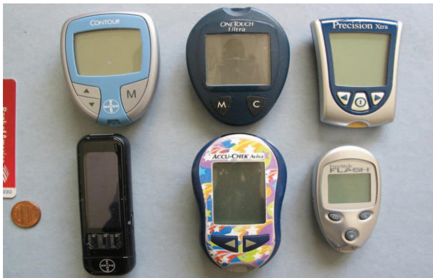
Figure 3.1 Commercially available enzymatic amperometric blood glucose monitoring Systems from major manufacturers (Bayer, Johnson and Johnson, Roche and Abbott, left to right, top to bottom).
