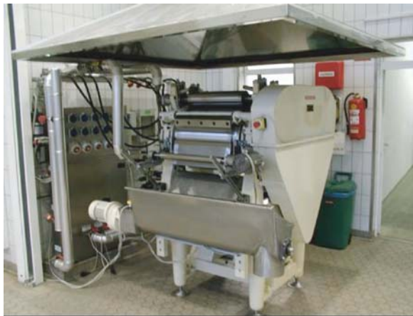
Figure 17.3. Drum dryer. (Pilot plant-University of Natural Resources and Applied Life Sciences)
