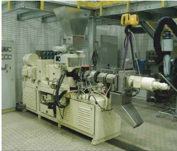
Figure 18.4. Extrusion cooker (Pilot plant – University of Natural Resources and Applied Life Sciences).
