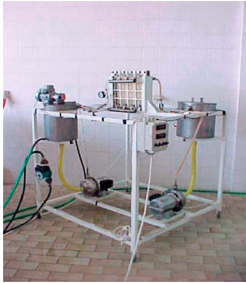
Figure 5.2. Experimental direct osmotic rig (Dova et al., 2006a).
