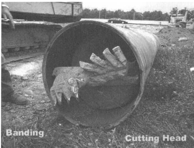
FIGURE 3. Sample Horizontal Auger Boring Cutting Head.
