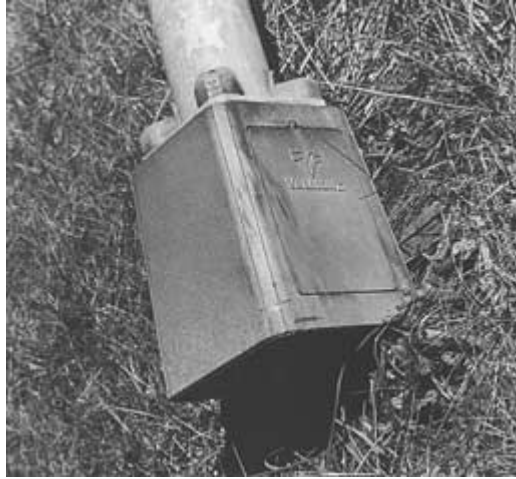
FIGURE 7.96 Separation of bottom flange from T-base.
