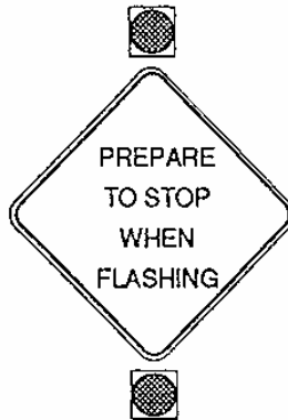
FIGURE 7.1 Example of supplemental advance warning sign.
