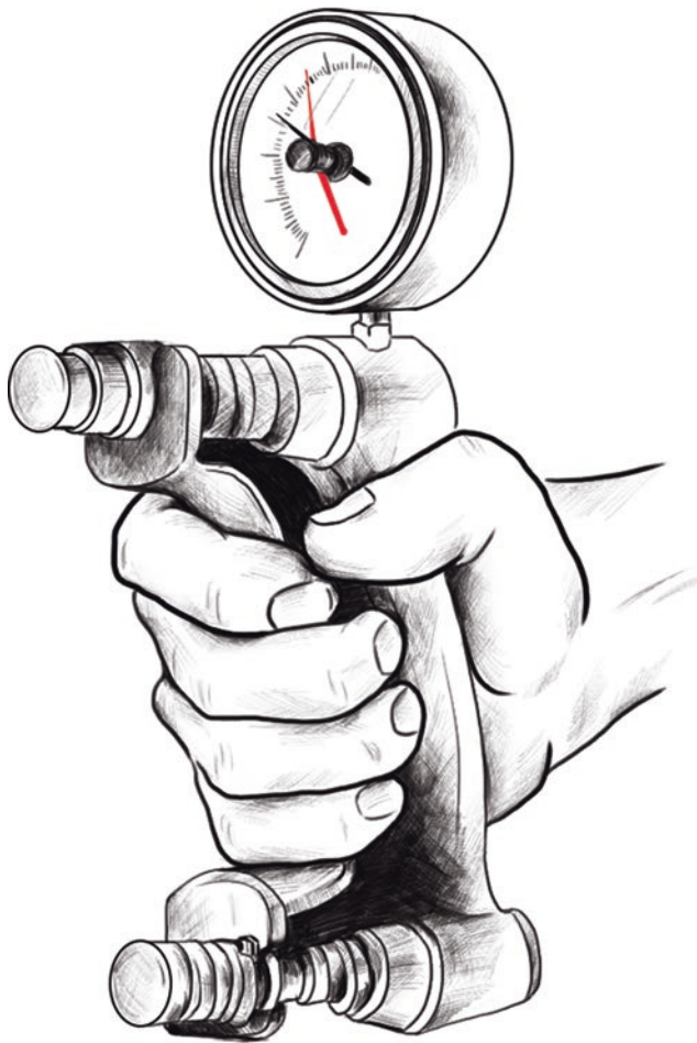
Fig. 2.39 The ergometer is used to measure the grip strength of the hands, and the results are accurate and reliable
