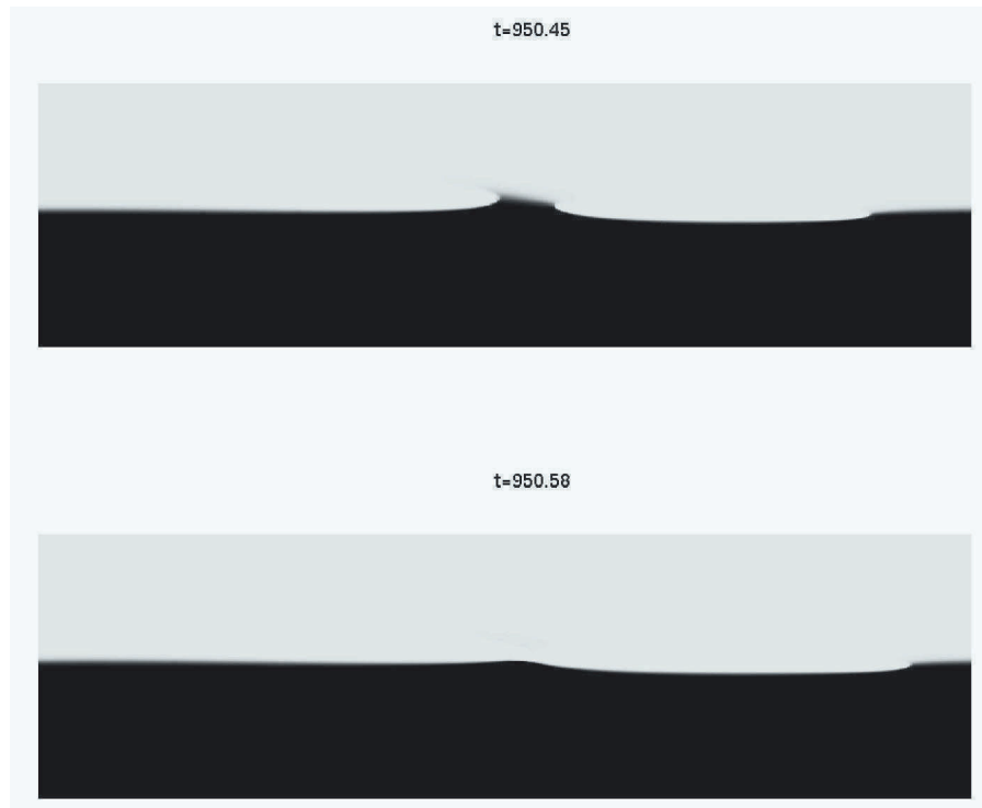
Figure 10. \eta as a function of \psi and z for selected times for ASCP solution with R = 7.5 . Axial direction is vertical.
