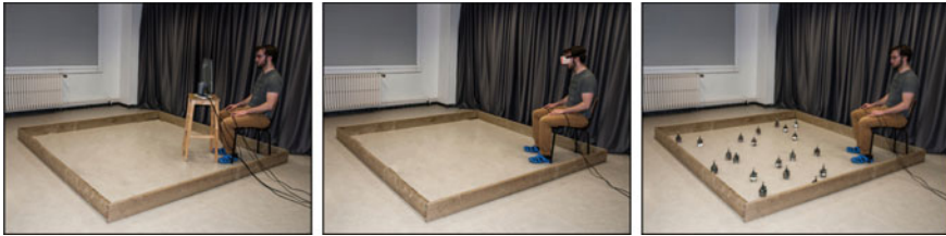
Fig. 1 Experimental scenario. Left: A participant interacts with a simulated swarm of 20 robots displayed on a computer screen. Middle: A participant is attached to a virtual reality head set and interacts with a simulated swarm of 20 robots. Right: A participant interacts with a swarm consisting of 20 real robots. The participant shown in this figure is the first author of this paper and did not take part in the experiment. The pictures shown in this figure were taken for illustration purpose
