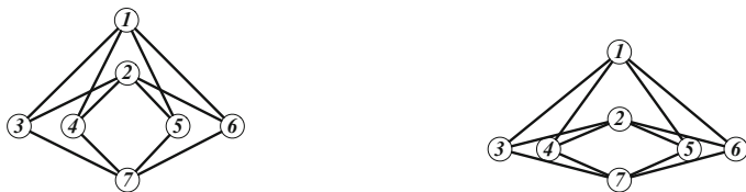
(a) A special geometric embedding with points on the x -axis and y -axis. (b) In this position, the framework is flexible.
