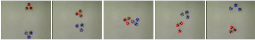
Fig. 7 Execution of the proposed algorithm in a scenario with 6 e-puck robots distributed in 2 groups
