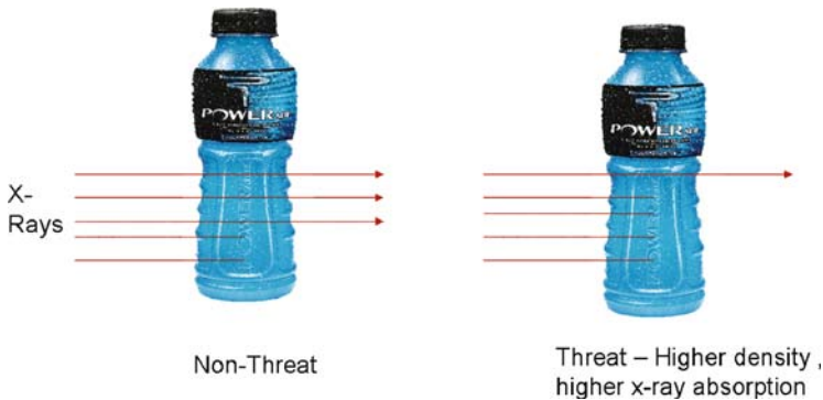
Fig. 5 X-ray interrogation principles
