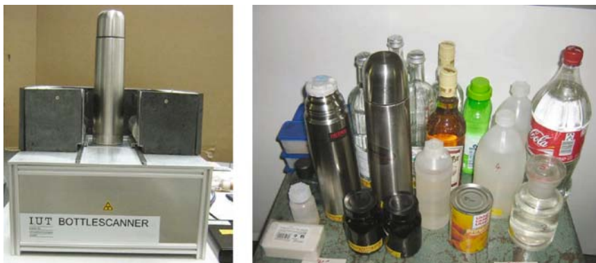
Fig. 13 BottleScanner for the liquid explosives detection and representation of inspected objects
