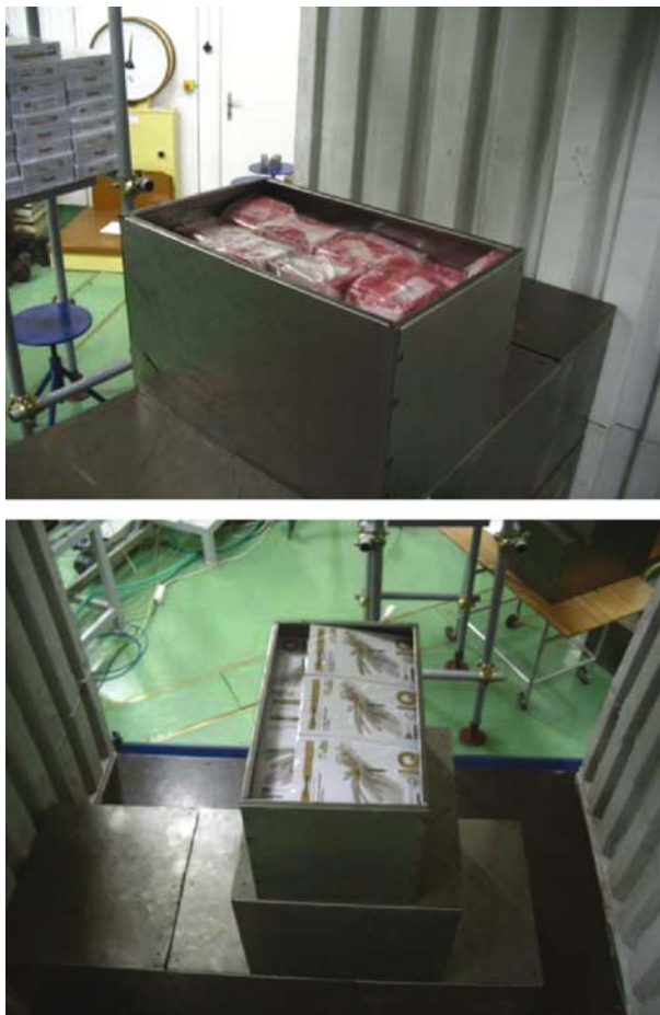
Fig. 7 Iron box full with the 100kg of the explosive Semtex1a (up) and iron box full with the 64.4kg of paper (down)
