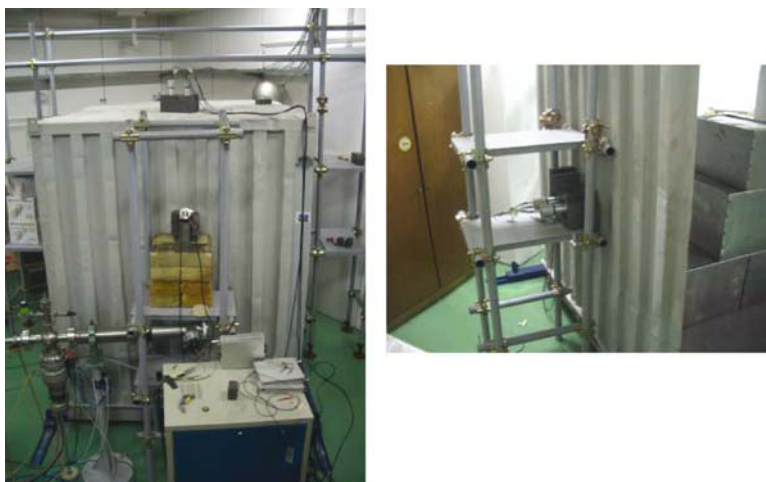
Fig. 2 Paraffine blocks over the neutron source and top detectors on the roof of the container (left) and transmission detectors (right)
