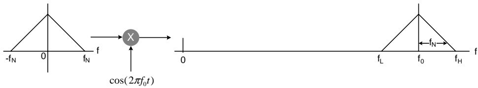
Figure 8.2 Baseband signal mixed with a carrier for signal translation in the frequency band
