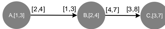
Figure 4.27 Example of a CSDFG, where node A first fires and takes 1 time unit and produces 2 tokens, and then in its second firing it takes 3 time units and generates 4 tokens. Node B in its first firing consumes 1 token in 2 time unit, and the in its second firing takes 4 time units and consumes 3 tokens; it respectively produces 4 and 7 tokens. A similar behavior of node C can be inferred from the figure
