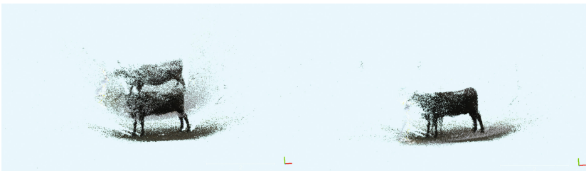
Fig. 8. PCD merged by two PCD of Fig. 7 without the alignment of ICP algorithm (left) and with the alignment of ICP algorithm (right).
