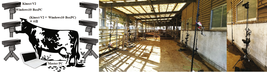
Fig. 2. Proposed system of 6 Kinect sensors.
