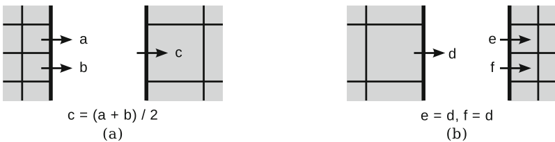
Fig. 4. Halo processing between different size of blocks. (a) fine to coarse. (b) coarse to fine.
