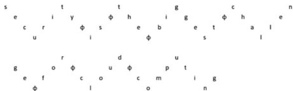
Fig. 9.1 Rail fence encryption with rail key 4
