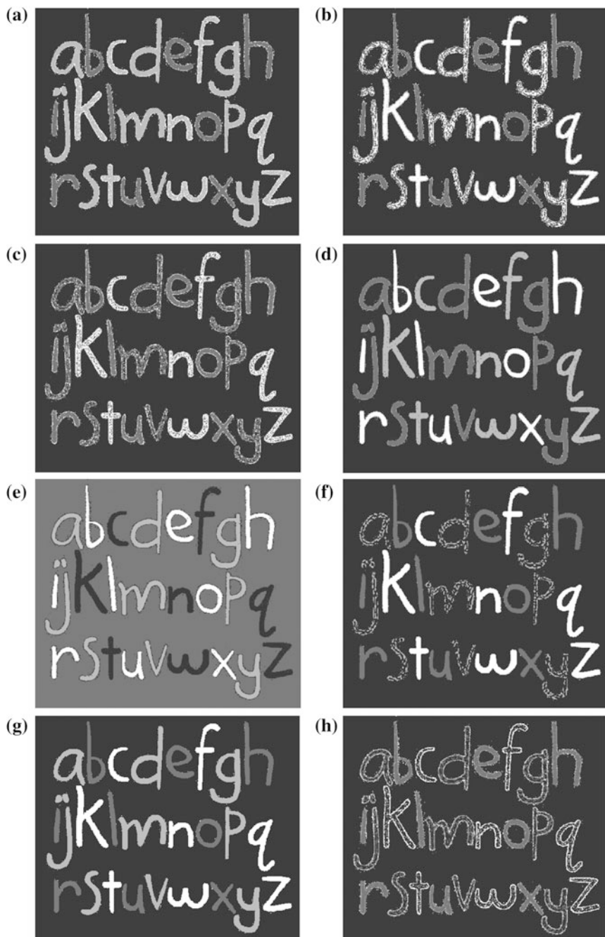
Fig. 9 a Clusters resulting from RGB. b Clusters resulting from HSV. c clusters coming from HSL. d Clusters coming from CIELab. e Cluster coming from nRGB. f Clusters coming from H. g Clusters coming from a fixed H component. h Cluster coming from HS
