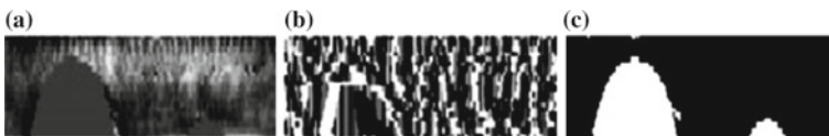
Fig. 9 Iris normalization and feature coding: a normalized image. b feature codes. c mask image
