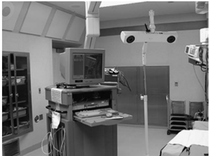
FIGURE 25–1. Computer workstation and optical camera array in the operating room. (StealthStation, Medtronic SNT, Louisville, CO)
