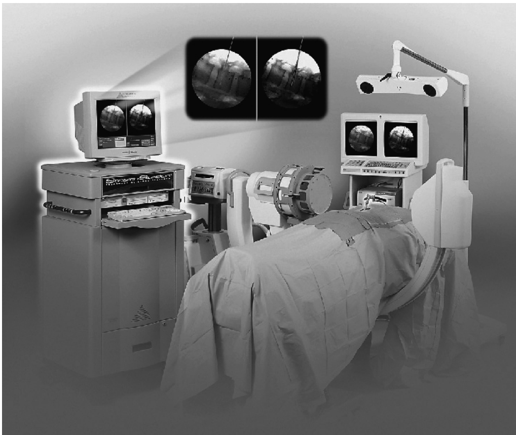
FIGURE 24–1. The FluoroNav (Medtronic SNT, Louisville, CO) virtual fluoroscopy system is shown, consisting of an image-guidance computer system and camera array, a calibration target that is attached to a standard C-arm fluoroscope, and various tracked tools. (From Foley KT, Simon DA, Rampersaud YR. Virtual fluoroscopy: computer-assisted fluoroscopic navigation. Spine 2001;26:347–351. With permission.)
