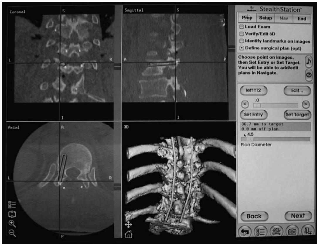
FIGURE 22–4. The intraoperative video of the spine at the image-guidance viewing station with the internal fiducials used as reference markers for obtaining accurate registration (StealthStation, Medtronic SNT, Louisville, CO).
