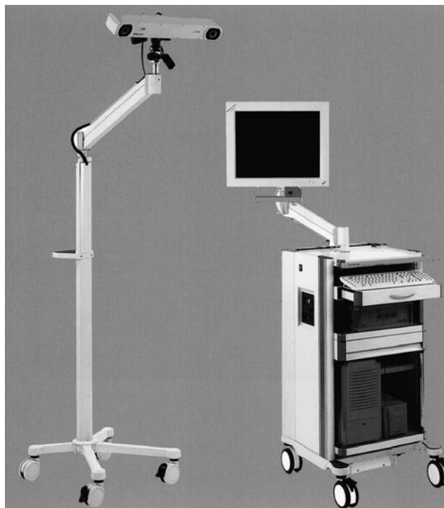
FIGURE 3-1. Image-guided navigational workstation with infrared camera localizer system.
