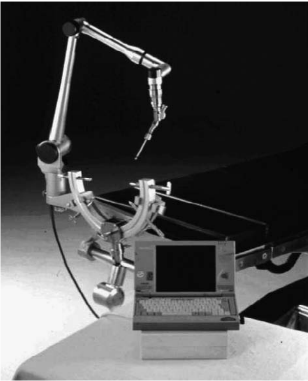
FIGURE 5-1. Basic construction of the neuronavigator, using a laptop PC running Microsoft Windows.
