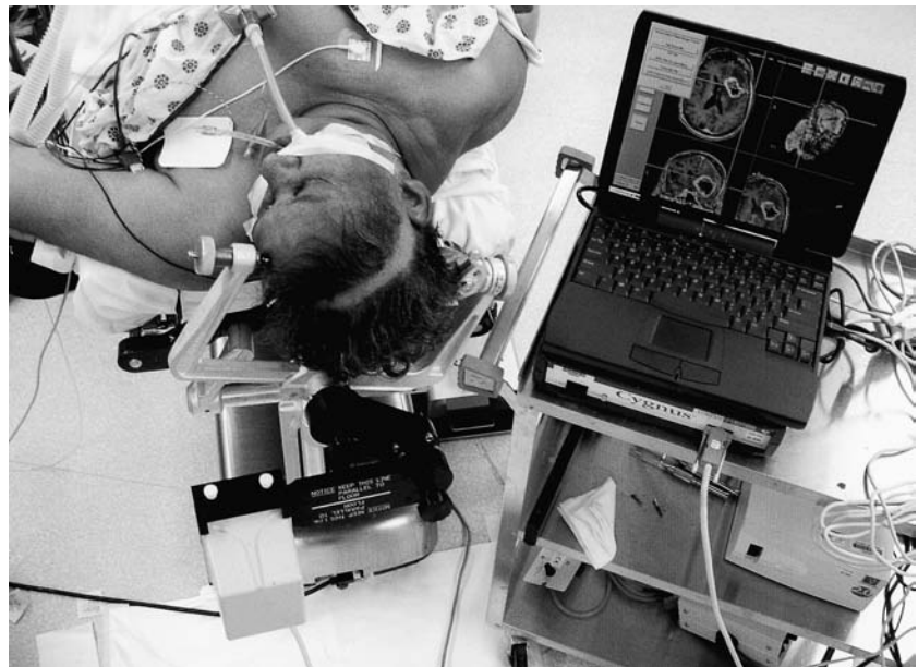
FIGURE 6–1. Cygnus-PFS setup for surgery illustrating magnet attached to head holder via L-shaped bracket, laptop computer, and magnetic control unit under computer (Compass International, Rochester, MN).
