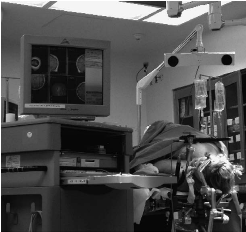
FIGURE 4-1. The computer workstation, optical digitizer, camera array, and reference arc demonstrating the intraoperative setup (StealthStation, Louisville, CO).
