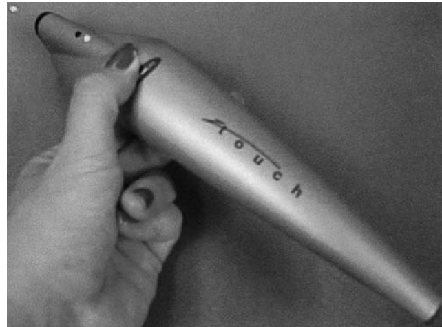
FIGURE 7-2. Z-touch registration instrument (BrainLAB, Redwood City, CA). This instrument can be used to register a patient in the operating room to images that do not have fiducial registration markers. The red laser beam emits an infrared beam of light that can be seen by the camera when the button (shown here) is pushed all the way down. This beam of light traces the structural features of the face, primarily picking out the bridge of the nose and the structures around the eye.
