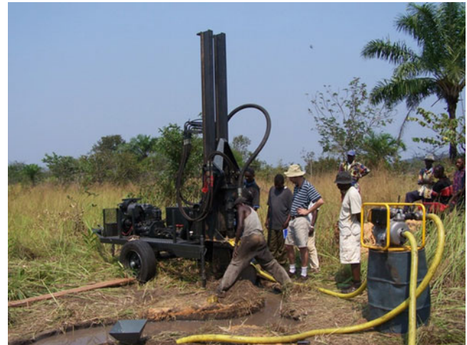
Fig. 16.14 Drilling operation on Kwango Terrace with a trailer-mounted Super Rock 100 (SR100) rig
