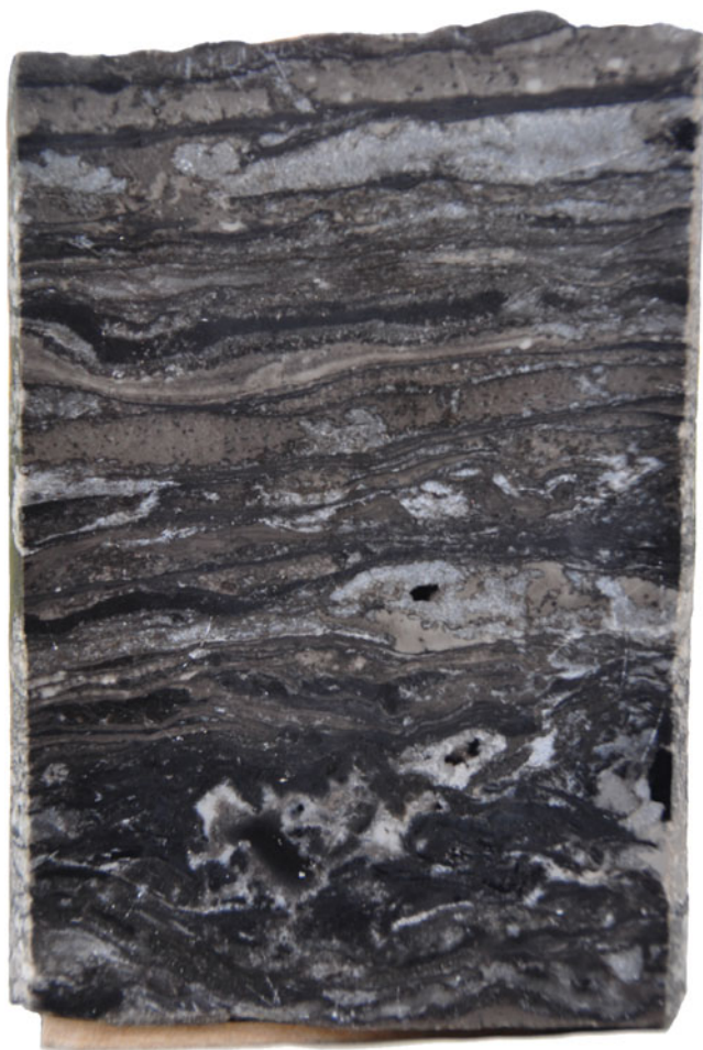
Fig. 7.5 Photo of drill core (No. 8) from the depth interval -4,139 m to -4,147 m in the Mbandaka-1 borehole. The cut face of the core shows thinly laminated (stromatolitic?) dolomitic fine sands and dark shales with large nodules of anhydrite. The core is 90 mm in diameter
