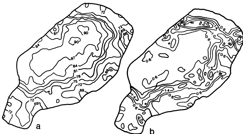
Figure 2 (a) Contour map of the Thornton and Tuttle Index over the Criffell pluton. (b) Approximation to the first derivative of (a) with values of less than 0.6 excluded
