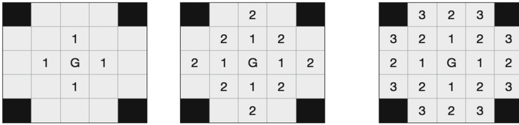
Fig. 2. Example of wavefront propagation.
