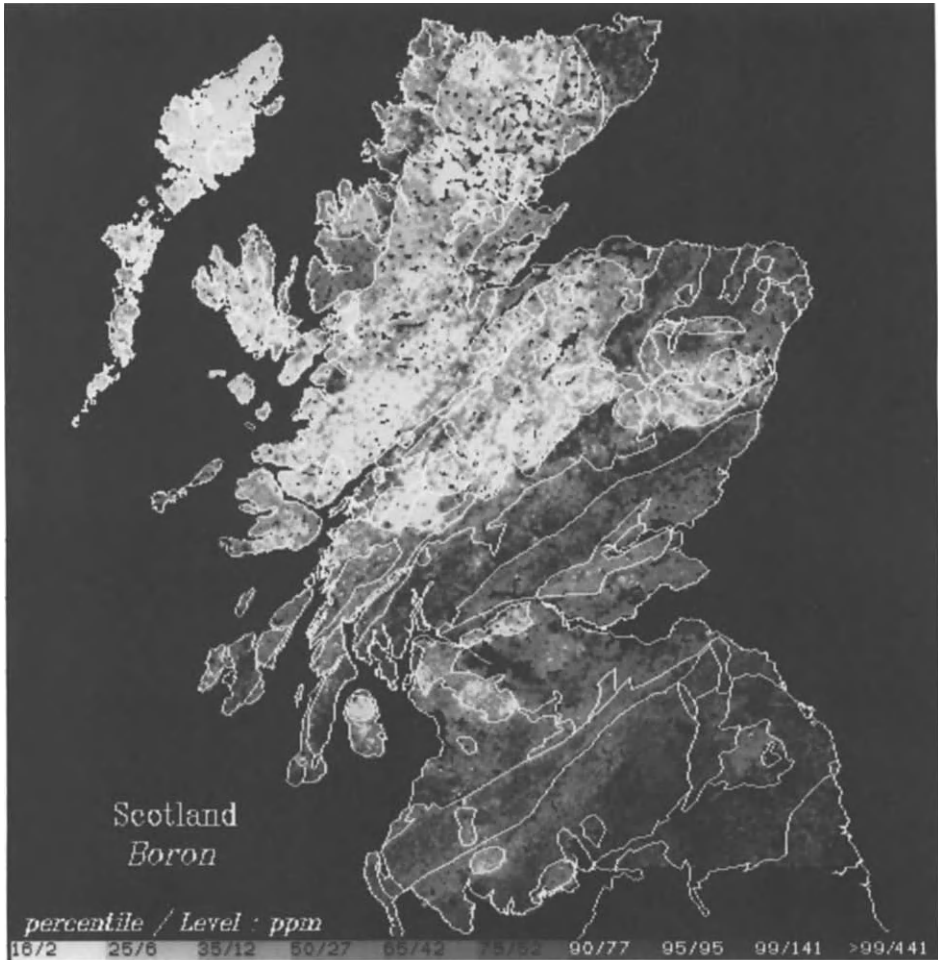
Fig. 4-12. Grey-tone geochemical map of boron in stream sediments in Scotland, with principal geological boundaries in white (courtesy of J.A. Plant).
