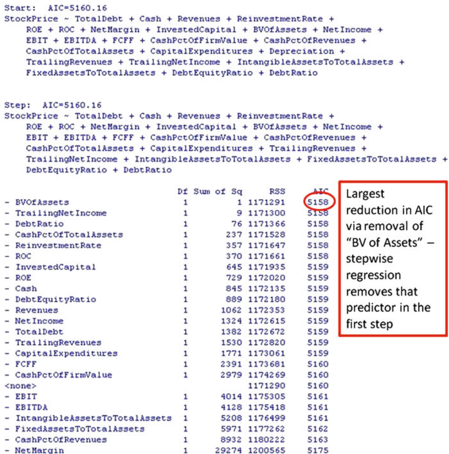
Fig. 5.10 First step of the stepwise regression procedure for the data in Table 5.3.
