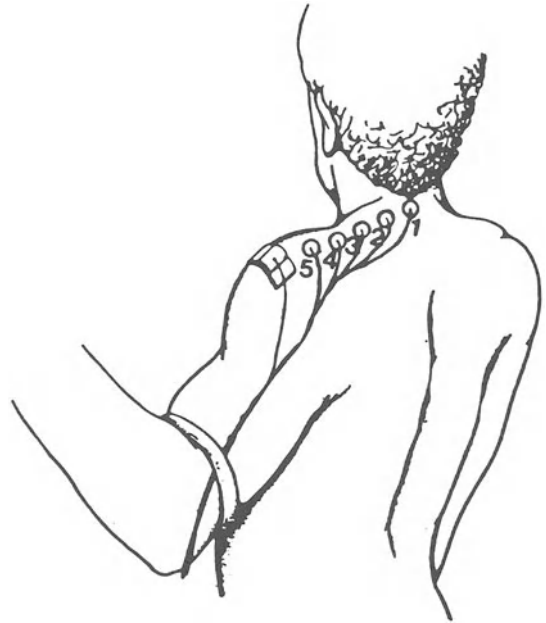
FIGURE 3.11. Five-electrode configuration on subject's shoulder used for sensory feedback for use with an FNS hand orthosis. (Reproduced from Riso and Ignagni, 1986, with permission of the Rehabilitation Engineering Society of North America.)
