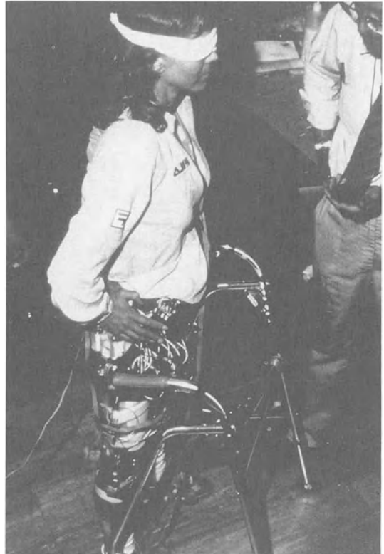
FIGURE 10.2. Paraplegic patient initially standing with the FES-orthosis and the sensory feedback system.
