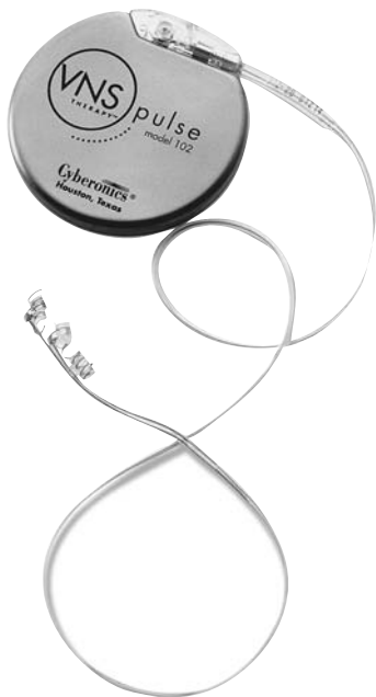
Fig. 13.3 Hardware showing pulse generator and lead. (From Cyberonics, Inc., Houston, Texas. Reprinted with permission.)
