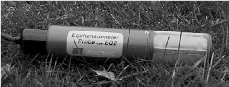
Fig 2. Equivalent Tensiometer – Equitensiometer EQT (Delta – T Devices, UK, 2000).
