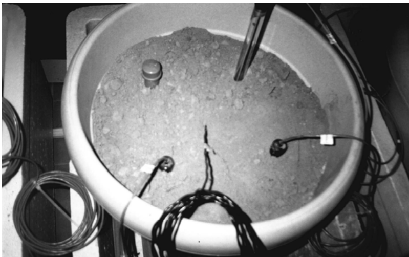
Fig 1. Mini-lysimeter and the instrumentation
