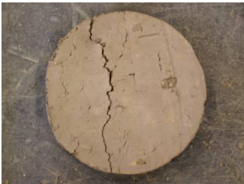
Fig. 1 A diametrical crack propagating across the sample associated with the “critical cracking ratio”
