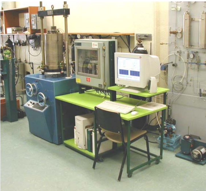
Fig. 1. Automated triaxial system with controlled suction
