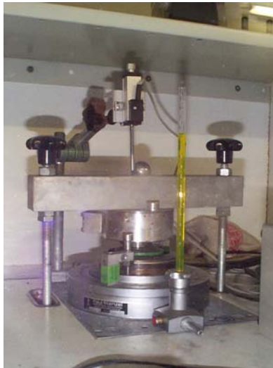
Fig. 4. Oedometer device with additional load cell
