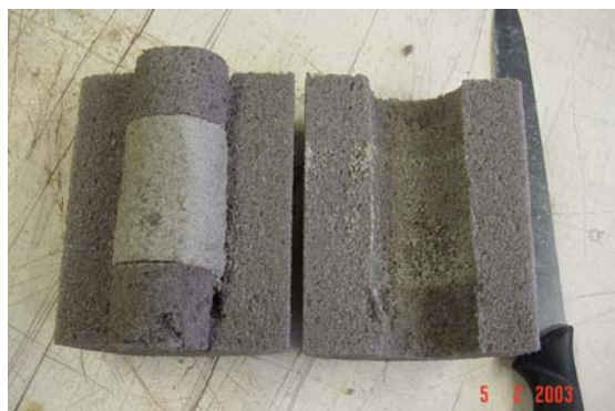
Fig. 6. Specimen in its “foam corset“ after test completion
