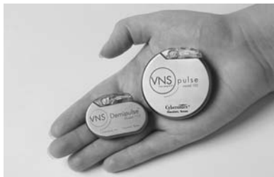
FIGURE 4.1 VNS therapy generators: model 102 (right side of picture) and 103 (left side of picture).
