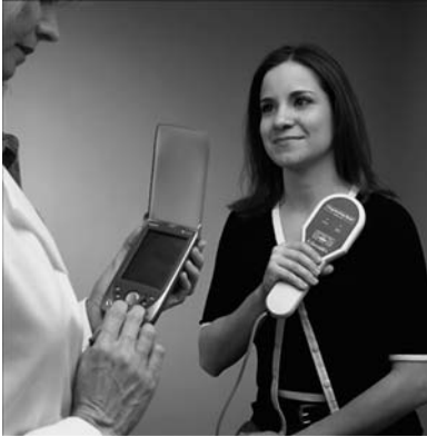
FIGURE 4.4 A programming wand is held by the patient over the device while a physician checks and/or adjusts stimulation parameters using a handheld computer.
