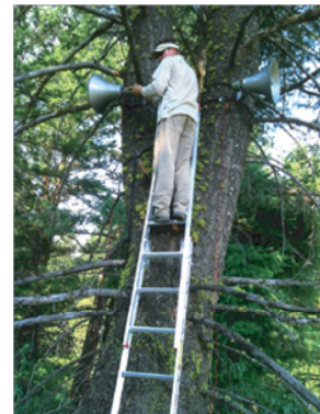
Figure 10.3 (A) Experimental set-up and background noise levels during the 'noise-on' phase of a manipulative experiment to test the effect of road noise on birds. The solid black line is a 500 m-long 'phantom road' (no paving, no traffic, just the loudspeakers) in a roadless area where migrating birds stop over in Idaho, United States. Road noise (higher db denoted in red, lower in blue) was propagated through 15 pairs of speakers (B, not shown on map) in 4-day intervals from 04:30 to 21:00, and the occurrence of birds was measured in the treatment areas (red squares) and control plots (green circles). Bird abundance was, on average, 22% lower at treatment plots and 12% higher at control plots, between noise-on and noise-off periods. Source: (A) Reproduced with permission of Christopher McClure and (B) Photograph by and reproduced with permission of Christopher McClure.
