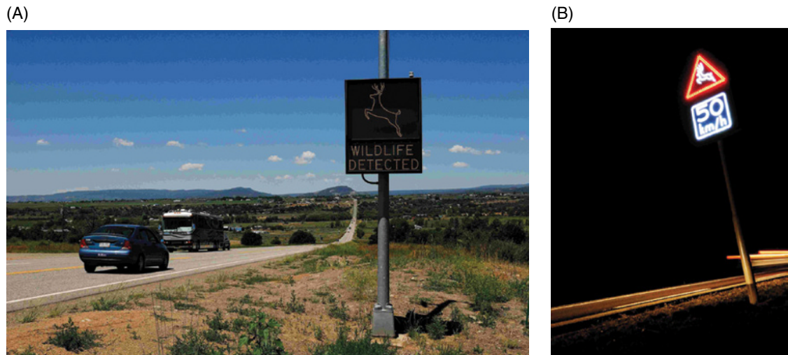
Figure 24.5 Activated warning signs on animal detection systems: (A) 'wildlife detected' Colorado, United States, and (B) activated warning sign and advisory speed limit reduction, the Netherlands. Source: Photographs by Marcel Huijser.
