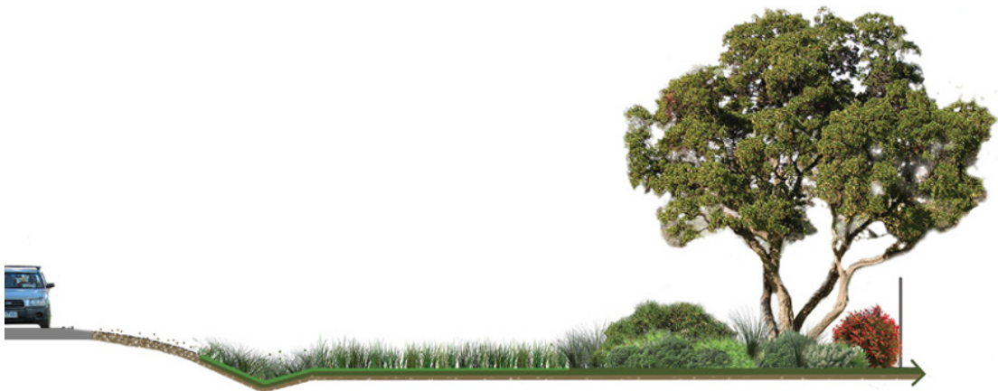
Figure 39.4 Schematic of road verge to provide habitat for small mammals, moving from longer grass within the clear zone through to shrubs and trees outside the clear zone. The size of each zone will depend on local safety standards and size of the right of way, and the exact mix of plant species and other structural elements (e.g. logs, rocks) will depend on the needs of the target species and maintenance requirements. Source: Reproduced with permission of Zoe Metherell.
