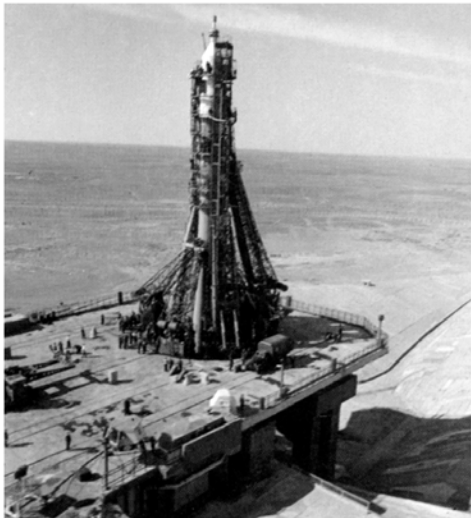
A Soyuz rocket is transported by rail to the launch pad, and installed in the support structure over the pit excavated into the Kazakh steppe.
