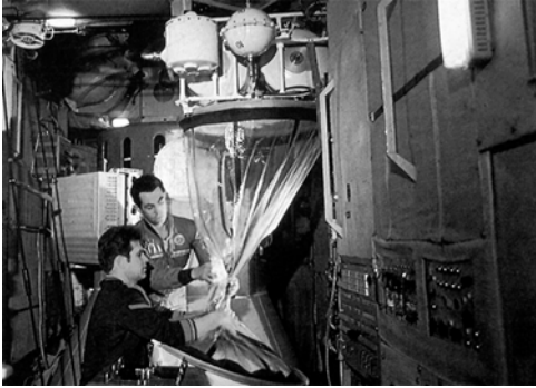
Vladimir Kovalyonok (left) and Viktor Savinykh prepare the shower in the Salyut 6 trainer, behind which is the conical bulk of the primary instrument.
