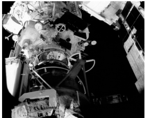
A view from STS-74 as the Docking Module is manoeuvred to mate with the axial port of the Kristall module.
