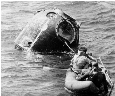
The Soyuz descent module is designed to float.
