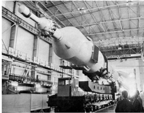
A view of Soyuz 18 in the assembly building, featuring its launch escape system.
