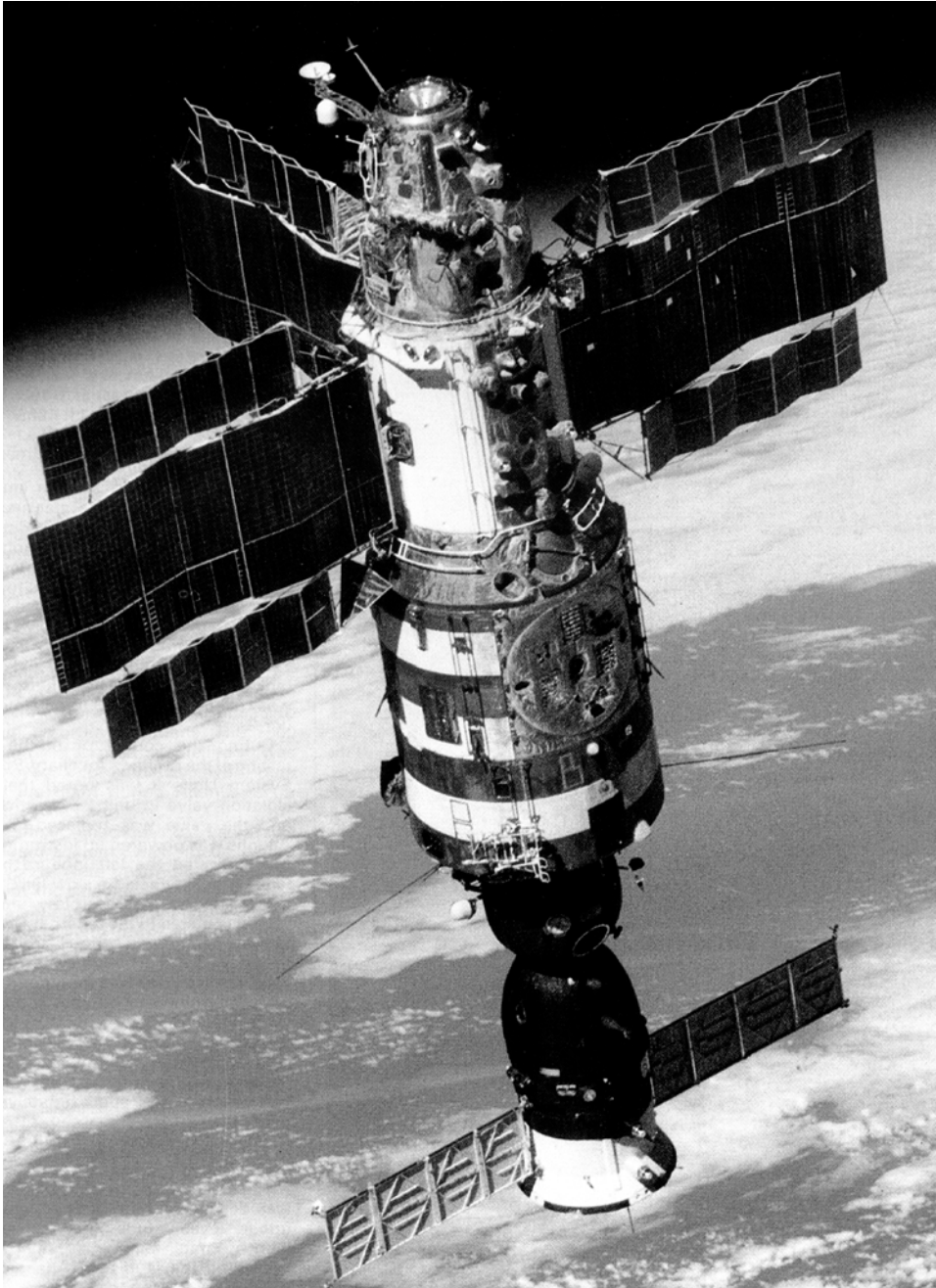
A magnificent view from Soyuz-T 13 of Salyut 7 with Soyuz-T 14 attached, and with a full set of clip-on solar panels.
