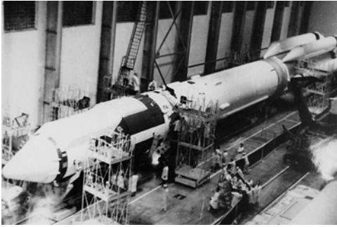
A Proton rocket with Salyut 2 protected by an aerodynamic shroud is about to be rolled out to the pad for launch.
