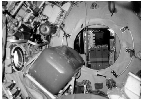
A view from Kvant 2's airlock through the inner hatch into its middle compartment, which served as an emergency airlock.
