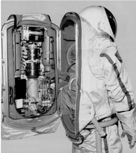
The rear hatch and integrated life-support backpack of the Orlan extravehicular suit.
