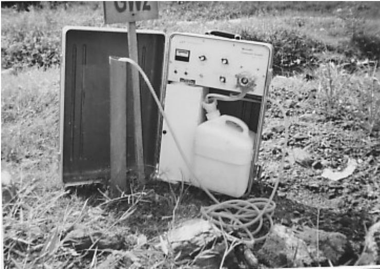
Figure 13. Abstraction of Groundwater Sample at GW2 Point. 9
