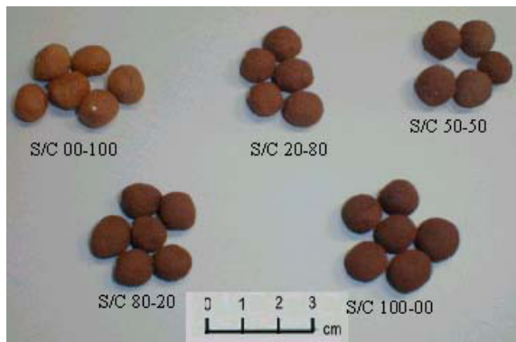
Figure 5. The Coarse Aggregates Made by Sintering Sludge/Clay Mixtures at 1,000°C.
