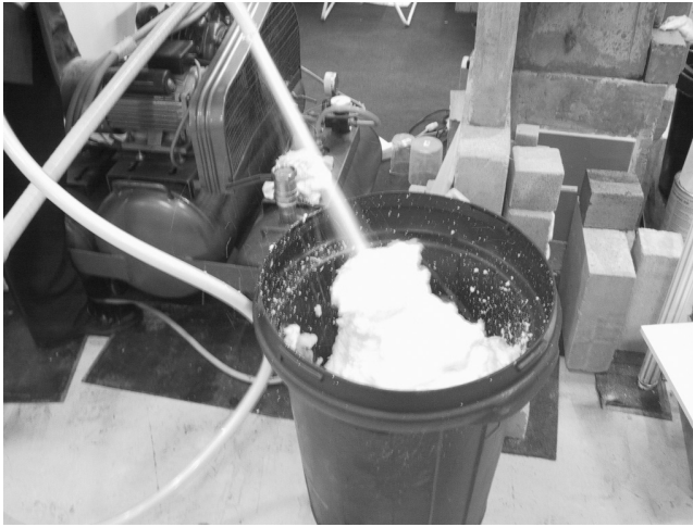
Figure 11. Experimental Foam Generation.
