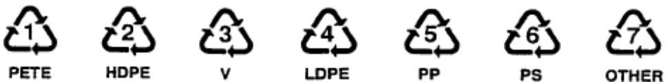
Figure 8. The American SPI Coding System. PETE: polyethylene terephthalate; HDPE: high-density polyethylene; V = PVC: polyvinyl chloride; LDPE: low-density polyethylene; PP: polypropylene; PS: polystyrene; Other: Other polymers or blends.
