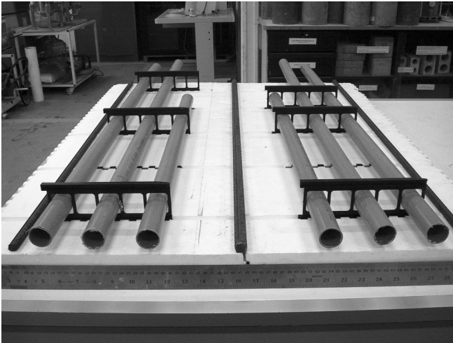
Figure 15. TIA Composite Web-PVC Pipe Reinforcement for Raised Floor System.
