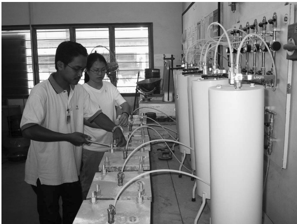
Figure 13. Testing for Water Permeability.
