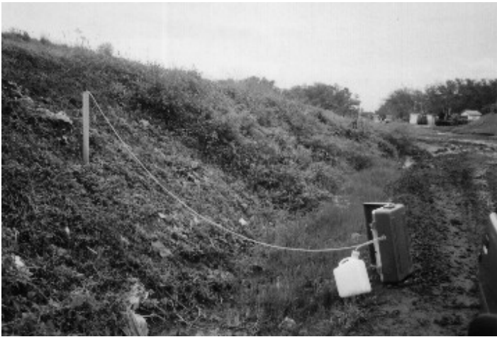
Figure 14. Abstraction of Groundwater Sample at GW5 Point. 10
