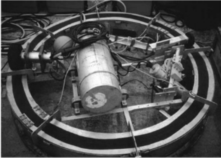
Figure 5. The Sea Carousel is a Benthic Annular Flume that is Used to Study the Effects on Increasing Current Flow on Sea-Floor Sediments.
