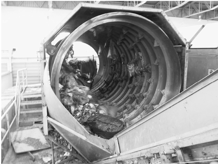
Figure 5. Trommel Screen for Waste Separation (a) Profile Diagram (11) and (b) Trommel Figure (Adapted from Taggart). 14
