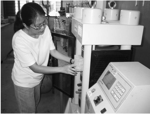
Figure 14. Testing for Compressive Strength.
